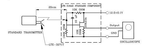
Fig. 3 Measuring method
